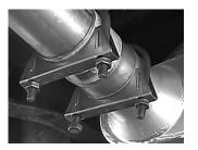
Step 2 Put on the clamp and nuts on
