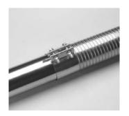
Manually fold the clamp ends to approximately 90 degrees. Insert foil gasket in gap and insert bolts into holes.
